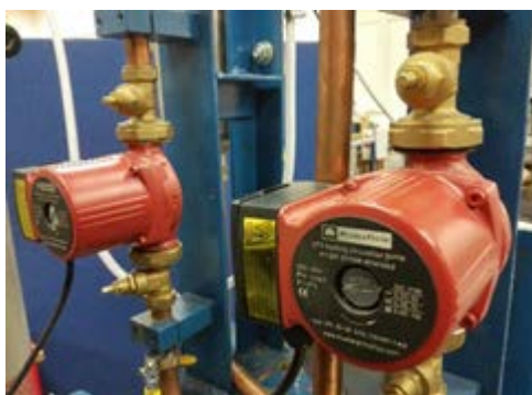
Figure 6.14 The pump employed in circulating system
