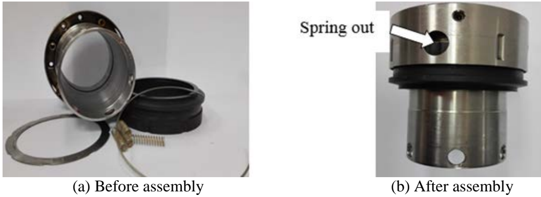
Figure 6.27 Seal head assembly in spring fault simulation
