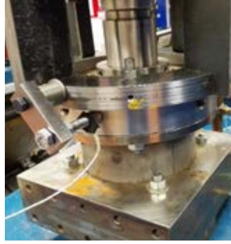
Figure 6.22 AE sensor mounted on the seal cartridge
