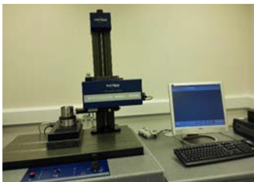
Figure 6.23 Taylor Hobson Form Talysurf applied in this research
