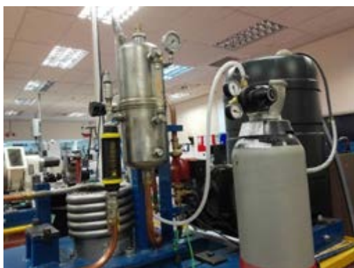
Figure 6.11 Multistage regulator mounted on the nitrogen cylinder
