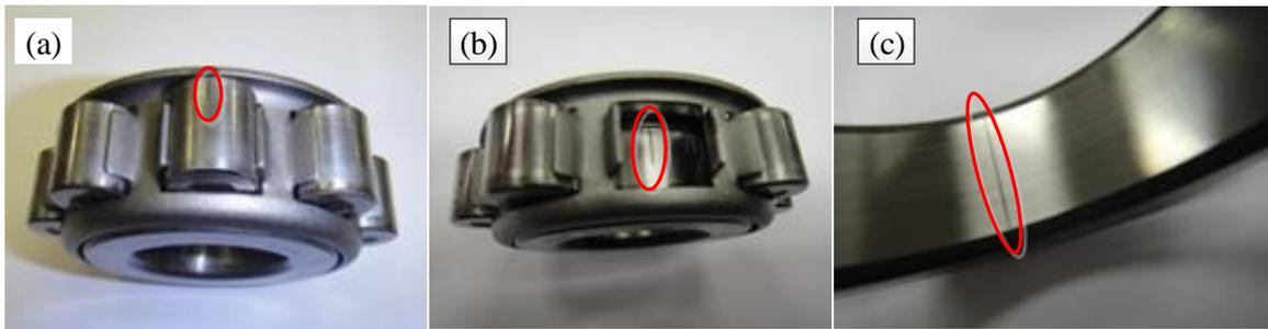
**Figure 6.10 Photographs of fault bearings**
